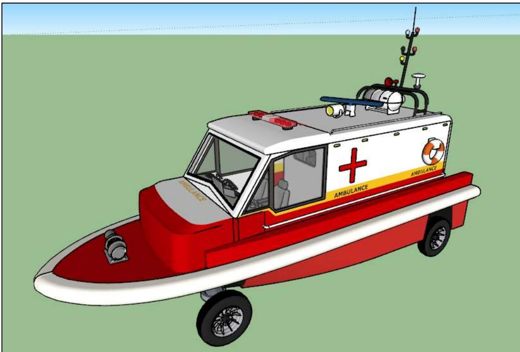
Gambar 6.7 Desain 3D *Amphibious HSAC* Mode di Darat
