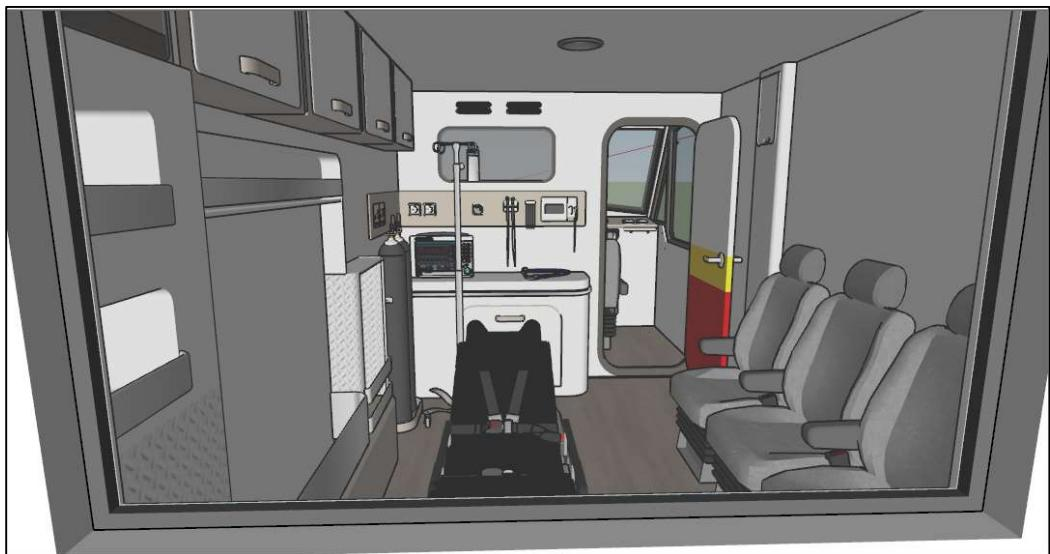
Gambar 6.9 Desain *Medical Compartment* 3D *Amphibious* HSAC
