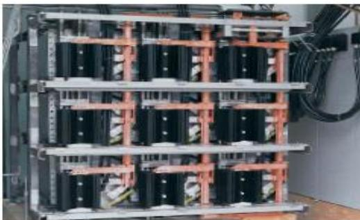
Fig. 12: PEM Fuel Cell modules assembled in a test rack
