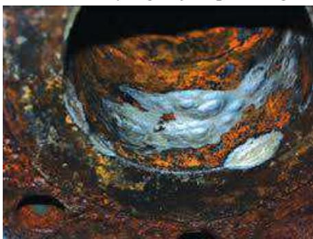
**Gambar 2.3 Internal Corrosion**
