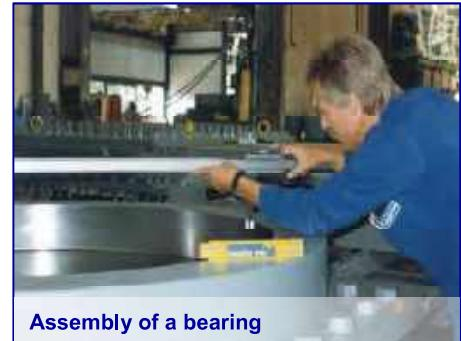
Assembly of a bearing
