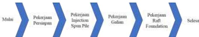
**Gambar 5. 25.** Alur Pekerjaan *Pile Raft Foundation*
