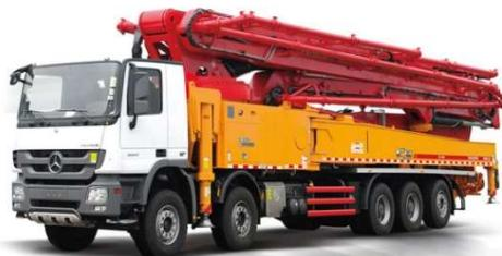
Gambar II.5 Concrete Pump
