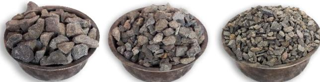
Gambar. 3.1 Agregat 10-20 mm ; 10-10mm ; 5-10mm
