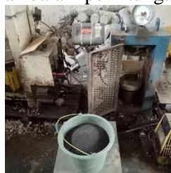
**Gambar 3.11** Menimbang Material Beton Geopolimer
