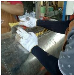
**Gambar 3.9** Menutup Mesin *Grinder* Semen Geopolimer
