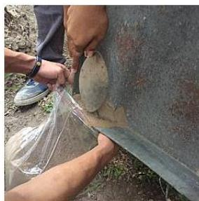
**Gambar 3.15** Mengemas Hasil Grinding Semen
