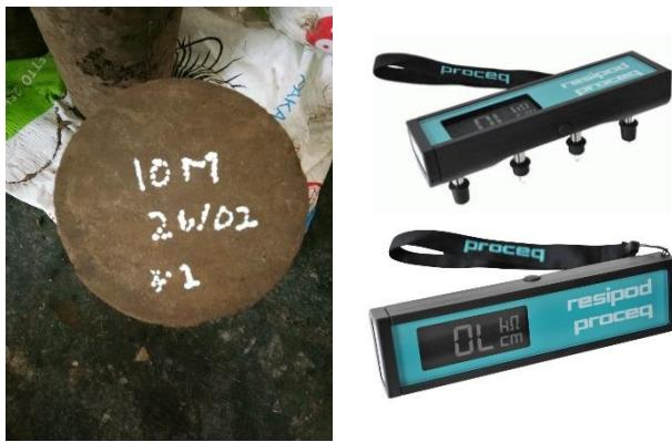
**Gambar 3.27** (a) Benda uji (b) Alat uji Resistivity
