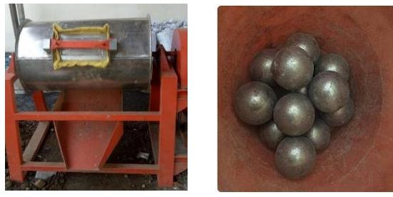
**Gambar 3.12** Alat Grinding; (a) Mesin Grinding (b) Bola Baja
