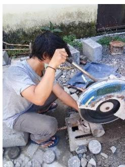
**Gambar 3.35** Memotong Benda Uji
