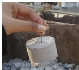
**Gambar 5. 10 Beton Decking Kolom**
