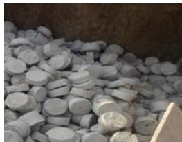
**Gambar 5. 16 Beton Decking *Shearwall***
