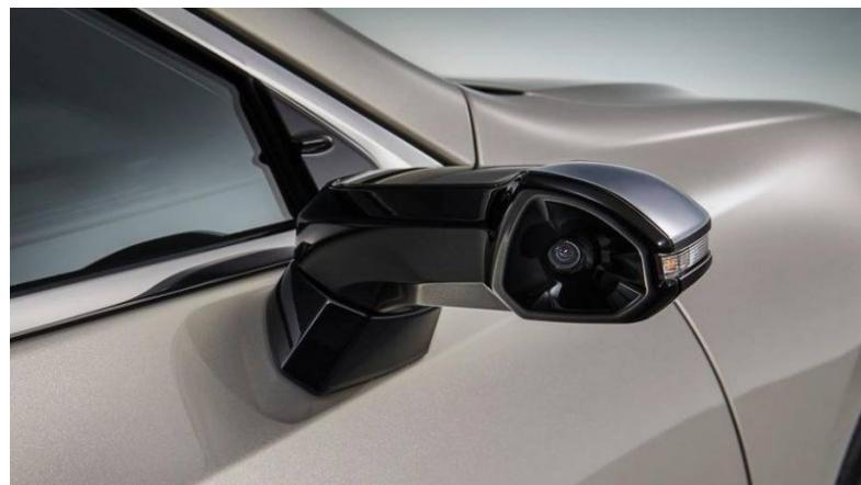
Gambar 2. 11. *Cameras Rear View Mirror*
