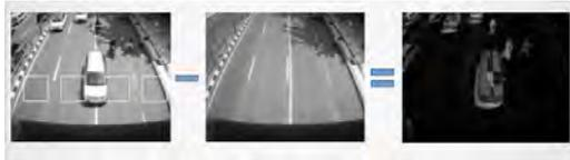
**Gambar 2.10:** Contoh proses *Background Subtraction*
