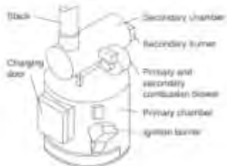
b.) Vertical two-chamber controlled air incinerator
