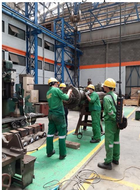
Proses Uji Contact Surface As Propeller
