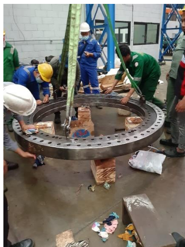
Proses perakitan bagian-bagian (part) Mean Ring Bearing
