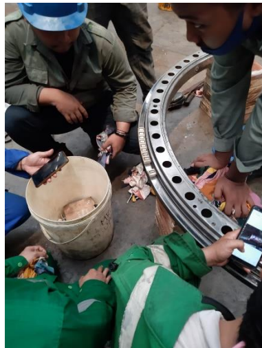
Pembersihan Mean Ring Bearing (MRB) sebelum perakitan (assembling)
