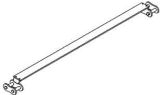
Gambar 4. 4 Rantai, *Attachment A2, Slat Chain Conveyor.*
