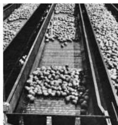
Gambar 2. 2. *roller chain slat conveyor.* ( *American Chain Association, 2006* ).
