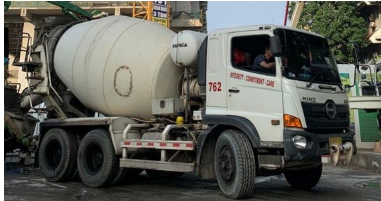
Gambar 3.7 Concrete Truck Mixer
