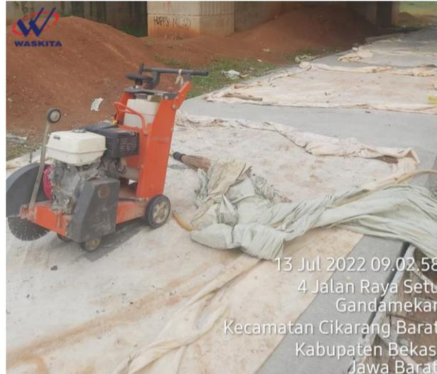
**Gambar 2.7** Concrete Saw Husqvarna FS400LV
