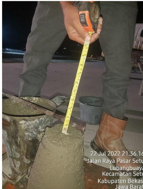
**Gambar 4.6** Proses Slump Test
