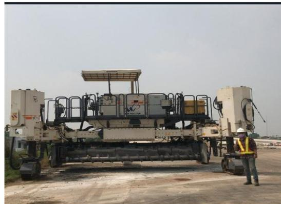
**Gambar 3.7** Concrete Paver
