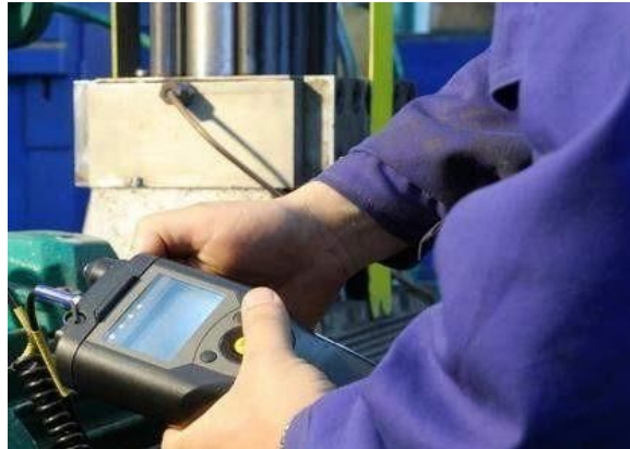
Gambar 4.49 Proses monitoring vibrasi
