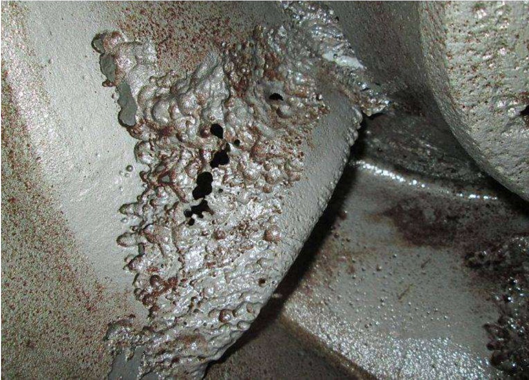
Gambar 4. 12 Kavitasi (sumber https://infimech.co.id/teori-kavitasi/ )
