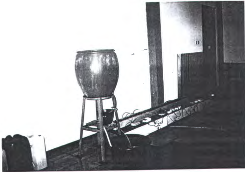
Foto 3. Reaktor Roughing Biofilter Horizontal
