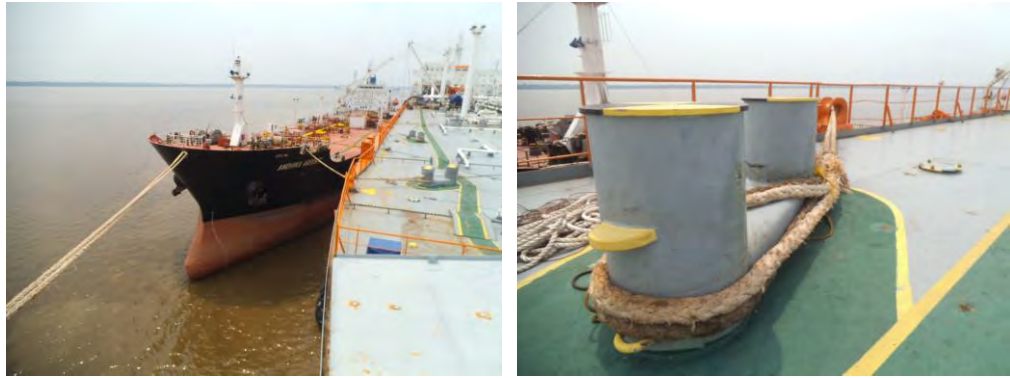
Gambar 2.1 Sistem offloading dan mooring system equipment di FSO Ladinda (Sumber: PT. Energi Mega Persada)
