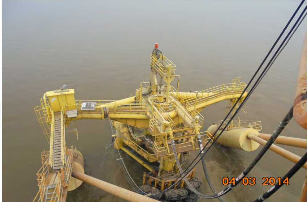
Gambar 1.2 mooring wishbone arm system attach to tripod SPOLS ( Single Point Offshore Loading System ) (Sumber ;PT. Energi Mega Persada)
