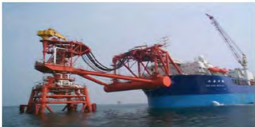
Gambar 2.8 Tower Yoke Mooring System (Sumber : Liu, 2007)
