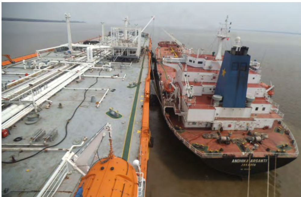
Gambar 1.3 side by side offloading process (Sumber ;PT. Energi Mega Persada)
