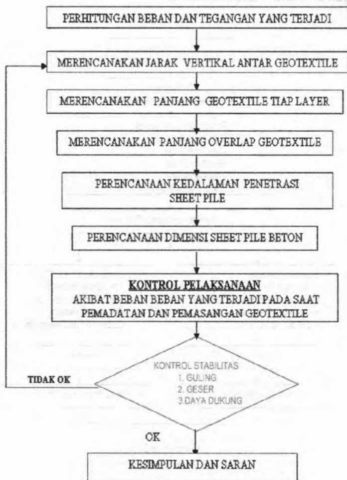
Gambar 3.2. Diagram Alir Kombinasi Sheet Pile - Geotextile
