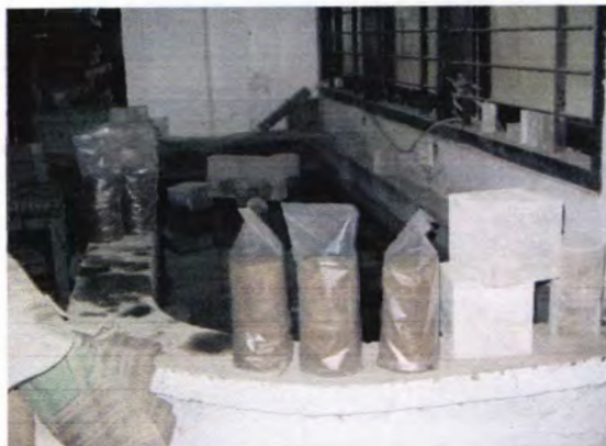
Gambar 3.21 curing suhu ruang beton geopolimer
