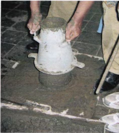
Gambar 3.22 Slump test beton
