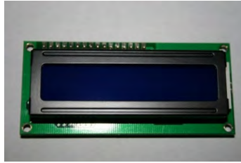
Gambar 2.6 LCD M1632 (Widodo, 2005)
