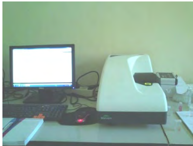
Gambar 3.3 Peralatan pengujian PSA ( Particle Size Analyzer ) di laboratorium zat padat, fisika, ITS Surabaya.
