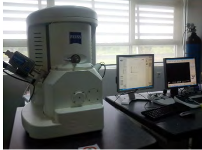
Gambar 3.2 Seperangkat peralatan SEM di laboratorium COE ( Center of Energy ) gedung robotika ITS Surabaya.
