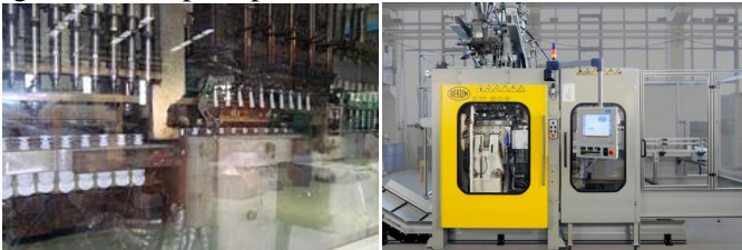
Gambar 2.9 Mesin blow molding PT. AAM
