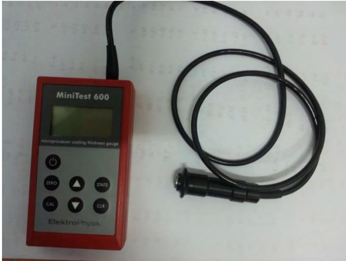
Gambar 2.6 Minitest 600 Microprocessor Coating Thickness Gauge
