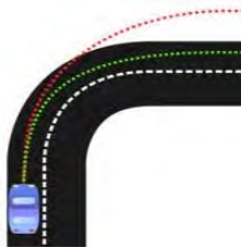
Gambar 2.13 Kendaraan mengalami understeer ( http://en.wikipedia.org/wiki/Understeer_and_oversteer )
