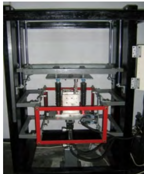
Gambar 3.22 Suspension Test Rig
