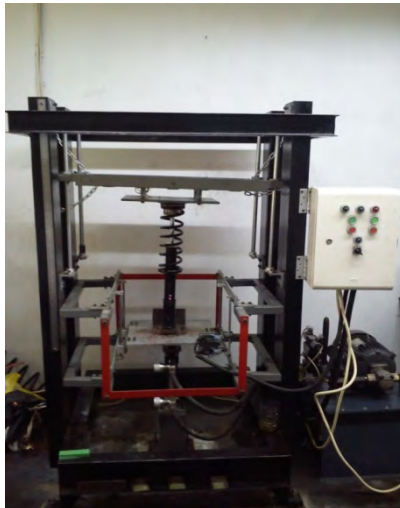
Gambar 2.9 Konstruksi Quarter car Suspension Test Rig ITS
