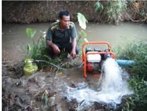
Gambar 1.1 Pompa Air LPG
