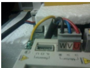
Gambar 4.27 Kabel motor servo AC ke driver motor
