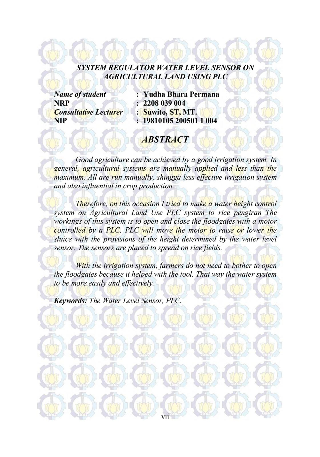
**SYSTEM REGULATOR WATER LEVEL SENSOR ON
