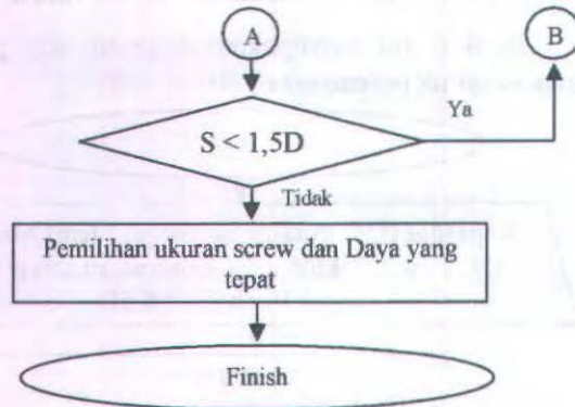
Gambar 3.3 Diagram Alir Perencanaan Screw Shaft
