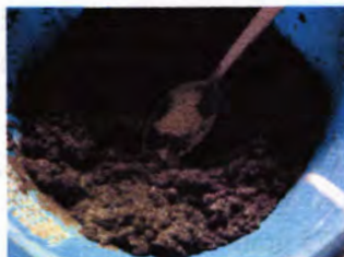
Gambar 4.18. Hasil campuran mortar trial mix 1
