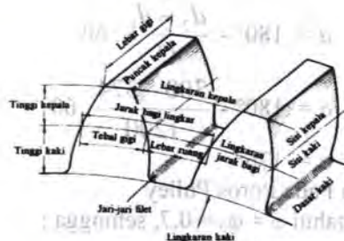
Gambar 4.14 Dimensi Spur Gear
