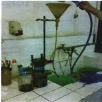
Gambar 4.4 Reaktor Constant Head Permeability Test
