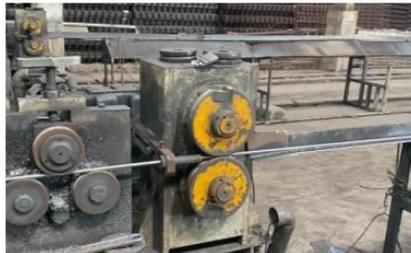
**Gambar 4.22** *Wire Cutter Machine*
