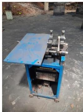
*Gambar 4.6 Mesin Butt Welding*
