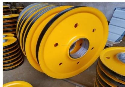
**Gambar 4.45** Pulley Crane
