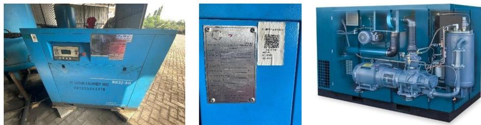
**Gambar 4.34** Screw Air Compressor
