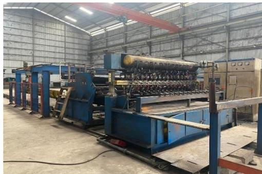
**Gambar 4.25** Welded Fabric Reinforcement Forming Machine di PT PIW
