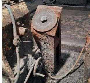
***Gambar 4.19 Feeder Drive Pulley***
