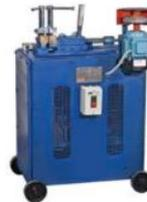
*Gambar 4.15 Mesin Butt Welding*
