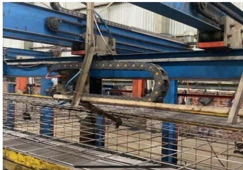
**Gambar 4.31** Griping Device For Welded Mesh
