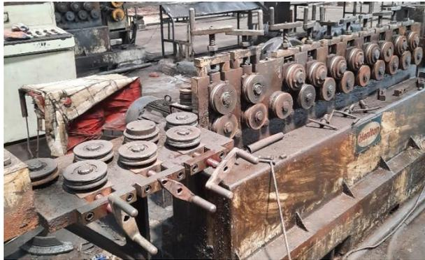
**Gambar 4.21** *Wire Straightening Machine*
