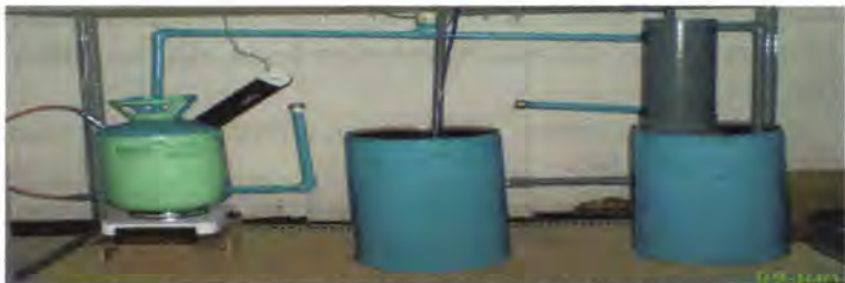
Gambar 4.1 Gambar Loop Pengendalian Pressure
