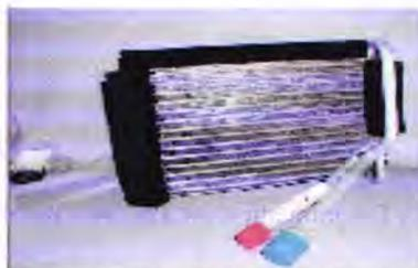
Gambar 2.5 Komponen Heat Exchanger
