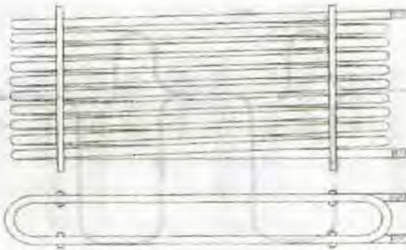
Gambar 2.12 Bare tube Evaporator jenis oval trombone coil
