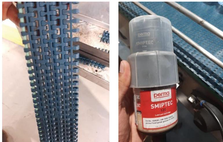
**Gambar 4.33** Pemasangan *Modular Belt* dan *Cartridge Automatic Lubricant*
