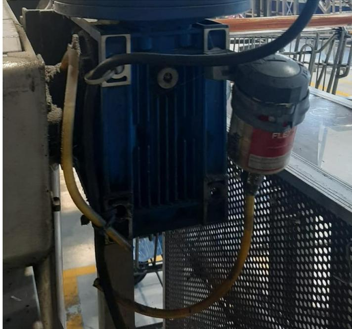
**Gambar 4.29** *Automatic Lubrication*
