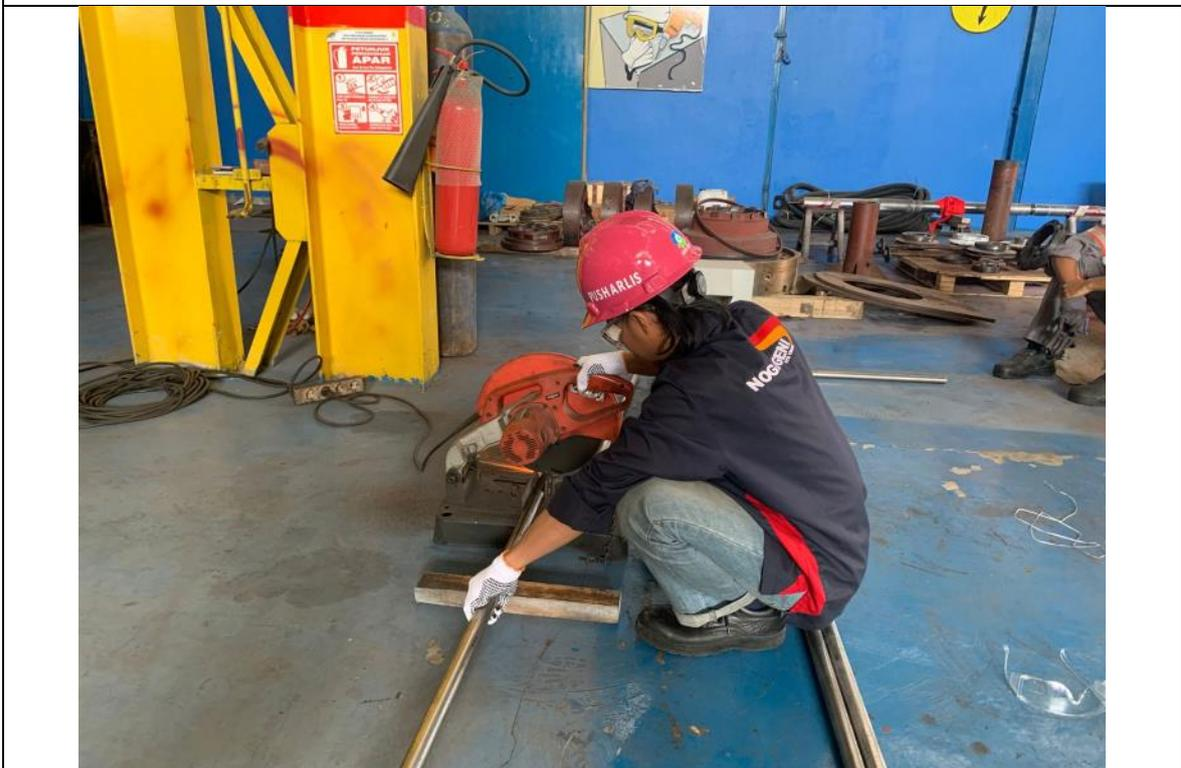
Memotong Stainless Steel Dengan Mesin Gerinda Tangan
