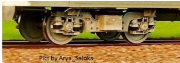
Gambar 4. 14 Bogie K-9 RE
