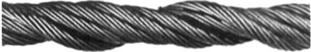
Gambar 4. 22 Thinning of The Rope (Kholis, 2014)
