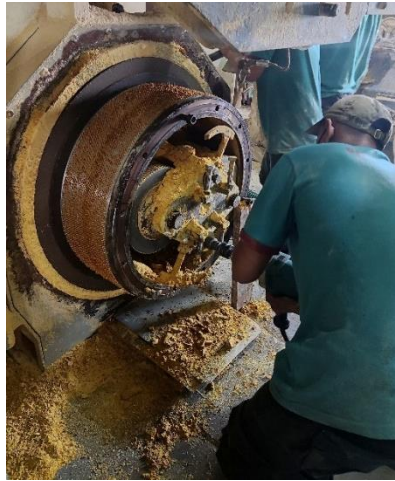
Gambar 4.38 Preventive Maintenance Pellet Mill
