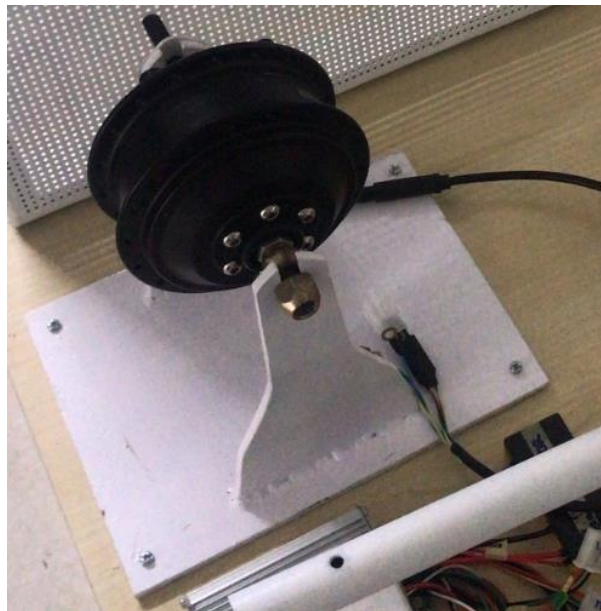
Gambar 4. 20 Mounting motor listrik
