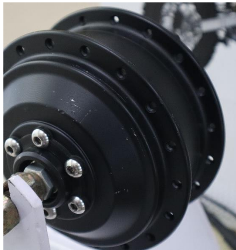
Gambar 4.4 Motor Listrik BLDC 350 WATT
