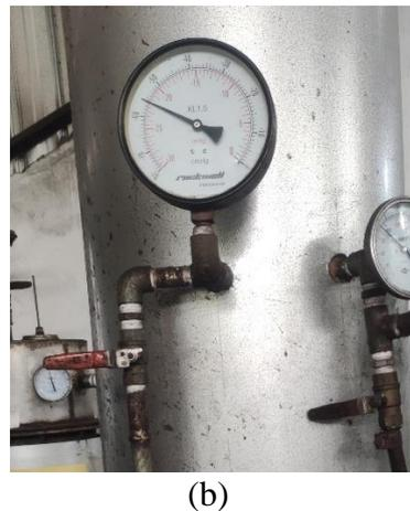
**Gambar 2.4** (a) Desain PFD Proses Evaporator dan (b) *Pressure Vacuum Gauge*
