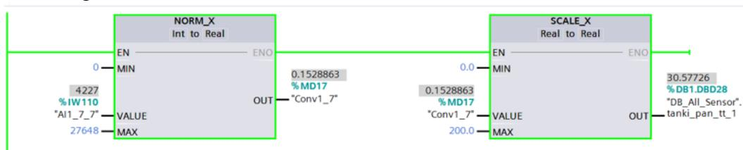
**Gambar 4.11** Program TIA Portal Unit Pan Masakan (Temperature)
