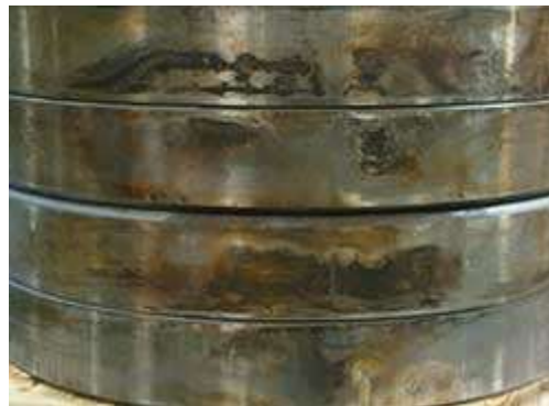
Gambar 2.12 Contoh fretting corrosion (Rosyidin, 2016)
