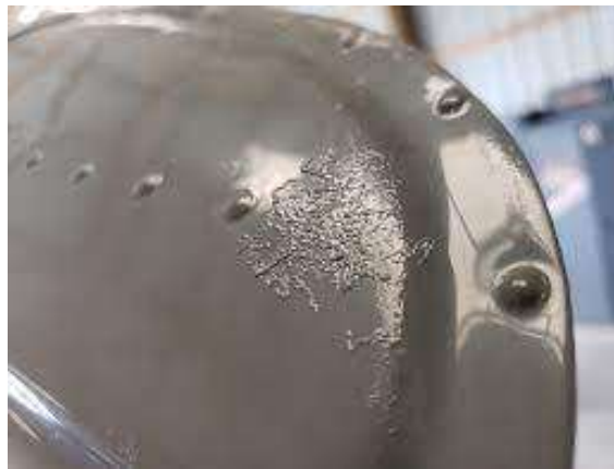
Gambar 2.13 Contoh filiform corrosion (Wahid, 1999)
